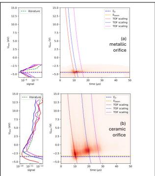
**Fig. 1**. Time-resolved IEDFs for a metallic (a) and a ceramic (b) orifice. The lines on the right panels indicate the shift due to the energy dependence of the time of flight in the MBMS.
